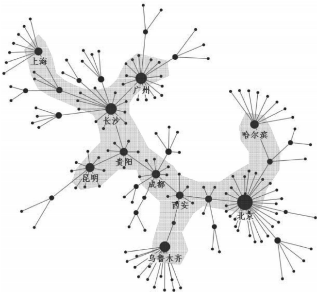
图8 中国城市航线网络的树形轴辐结构拓扑图 Fig. 8 The tree hub-spoke topology structure of Chinese aviation network
