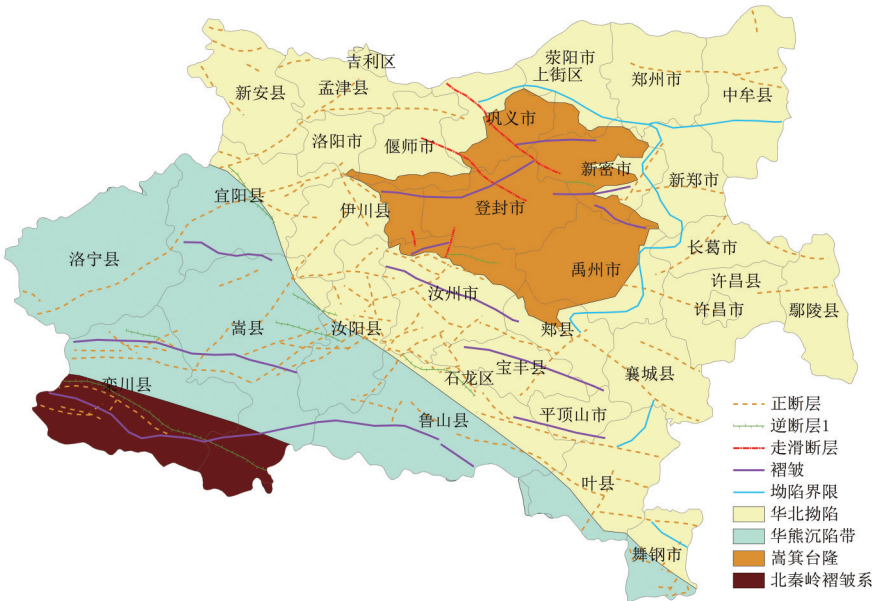
图2 环嵩山地区构造示意图 Fig. 2 The tectonics around Songshan Mountain
