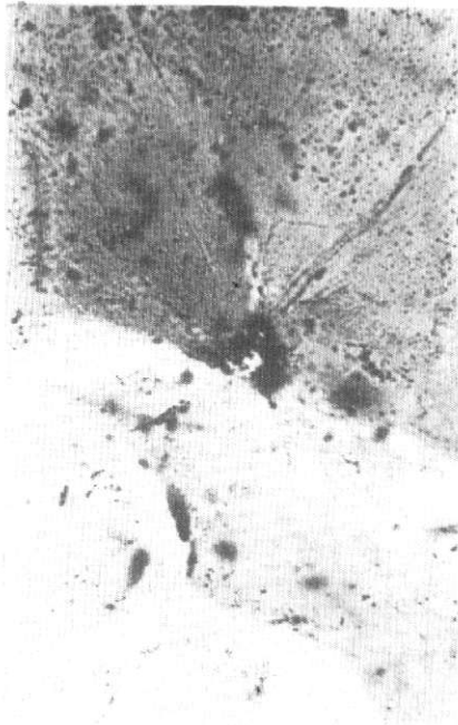
照片 8 柯石英相转变产生的放射状裂隙(两颗石英之间), 黑色为震变玻璃。正交 \times 250 。 Photo. 8 Radial fissures created by the phase transforma- tion of cosite to \alpha -quartz occurred between two quartz grains (Black parts are diaplectic glasses).
